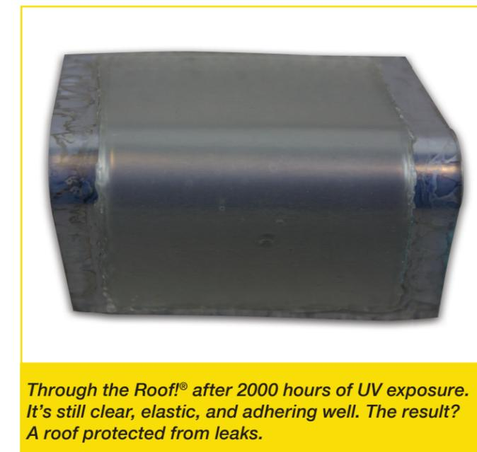
Through the Roof!<sup>®</sup> after 2000 hours of UV exposure. It's still clear, elastic, and adhering well. The result? A roof protected from leaks.
