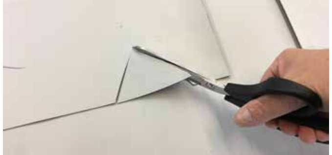
Leister scissors with special serrated edge for complex requirements when cutting plastic sheets.
