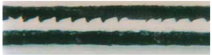
Welded with grip nozzle 25% higher weld seam strength. Mainly for TPO sealing sheets.
