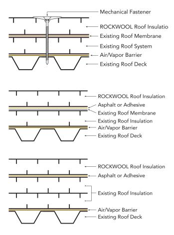
When installing multiple layers of insulation, good roofing practice recommends staggering the joints a minimum of 6".
