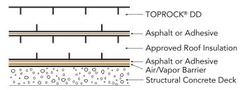
When installing multiple layers of insulation, good roofing practice recommends staggering the joints a minimum of 6".
