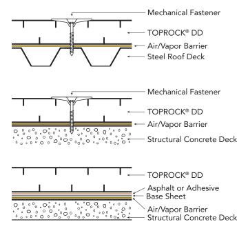
When installing multiple layers of insulation, good roofing practice recommends staggering the joints a minimum of 6".
